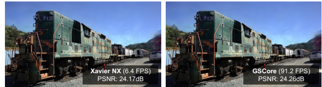
Figure 1. Rendering with 3D Gaussian Splatting [25] on Jetson Xavier NX and GSCore. The rendered image for GSCore is obtained from our simulator. The model is trained for 30K iterations.
